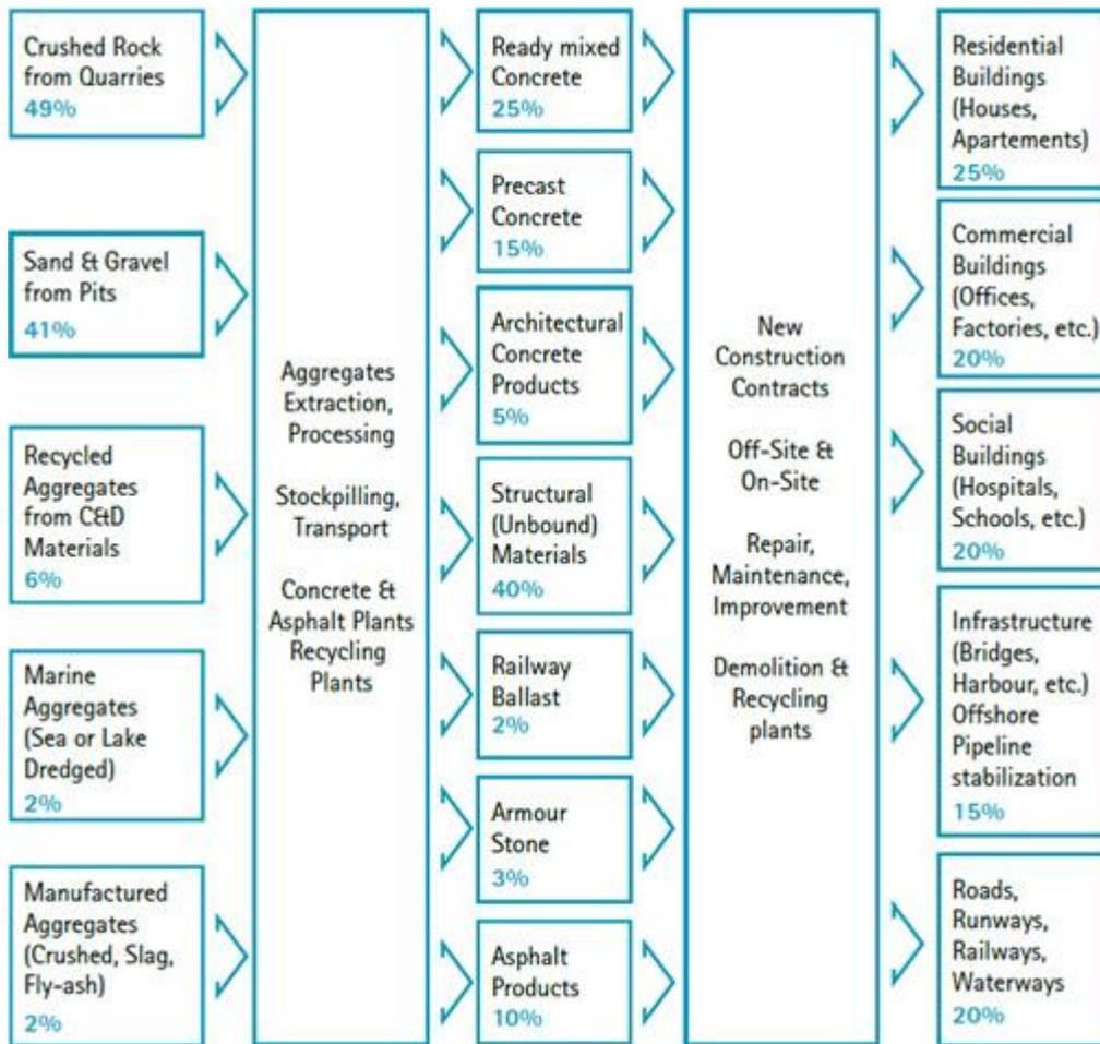
Figure 2 - Sourcing, Production and Use of Aggregates in Europe (UEPG, 2014b)
